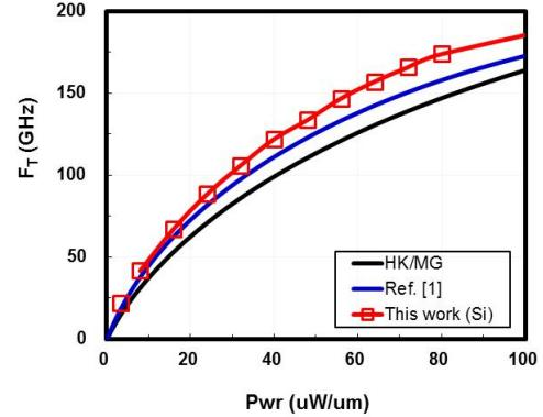
Fig. 6 NMOS RF cut-off frequency ( $f_T$ ) vs. power at  $V_{gs}=0.5\text{V}$  and  $V_{ds}=0.8\text{V}$ .
