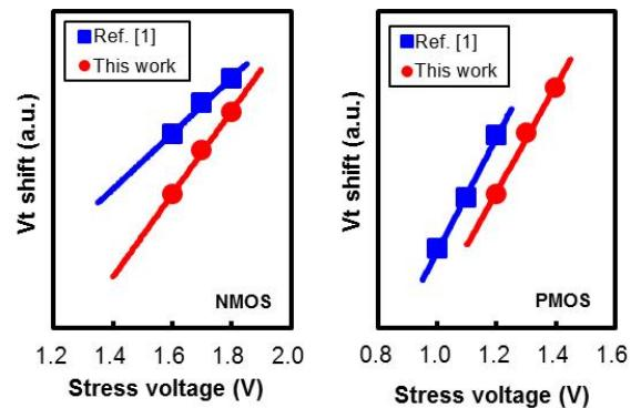
Fig. 14 Improved core device NBTI and PBTI in this work.
