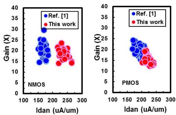
Fig. 4 Core device intrinsic gain (gm/gds) vs. drain current at  $V_{gs}=V_t+200\text{mV}$  and  $V_{ds}=0.5 \times V_{dd}$ .
