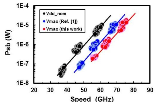
Fig. 16 The improved Vmax provides additional 10% R.O. speed gain.
