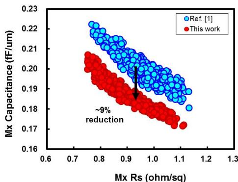
Fig.11 Metal capacitance is reduced by ~9% for Mx pitch of 64nm.
