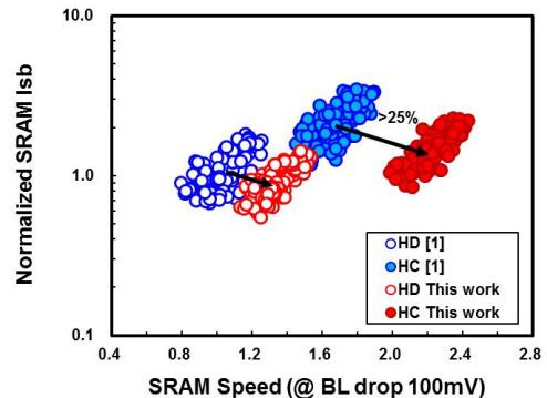
Fig. 8 HC/HD SRAM cell speed is boosted by >25% with less lsb.
