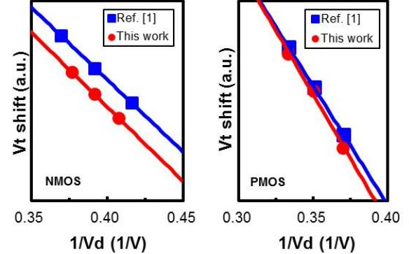
Fig. 15 I/O NMOS and PMOS HCI are improved by S/D junction opt.
