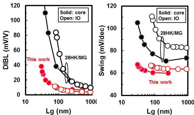
Fig. 3 Superior FinFET device DIBL and sub-threshold swing.
