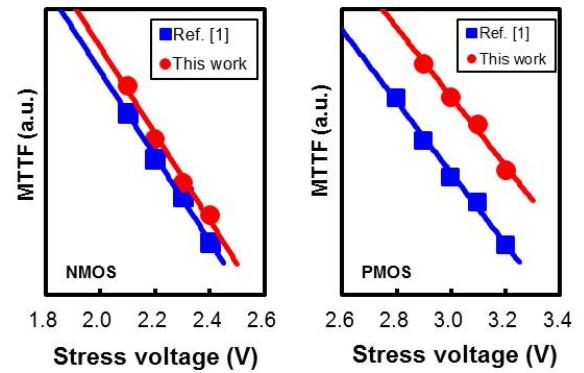
Fig. 13 Improved core NMOS and PMOS TDDB in this work.
