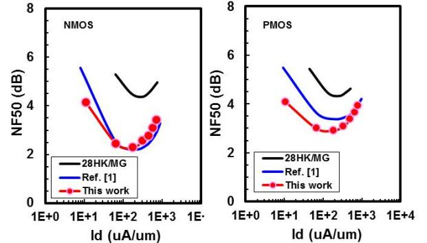
Fig. 7 FinFET devices achieve lower thermal noise than 28HK/MG.
