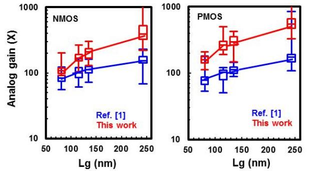
Fig. 5 Improved I/O device intrinsic gain (gm/gds) vs. Lg.
