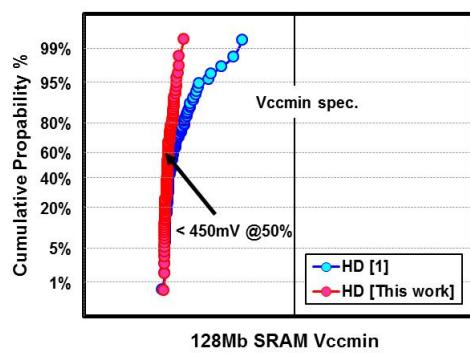
Fig. 10 128Mb HD SRAM Vccmin capability of 450mV is achieved.
