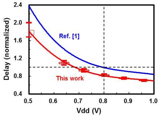
Fig. 2 CV/I of an inverter R.O. (F.O.=3) at different Vdd.
