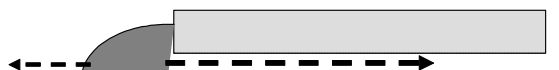
Figure 14: Competing forces for underfill spread under the die vs. away from die
